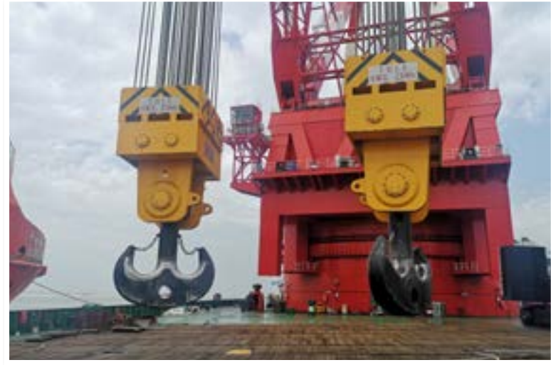
2020年，4600T海上风电施工船“冠盛一航”号采用两套2300t吊钩组由新华起重工具提供 In 2020, "Guan Sheng Yi Hang" floating crane (4600t) 2 sets of hook blocks are provided by THLE.
